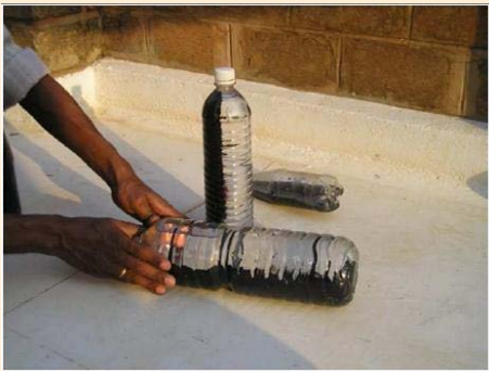
Picture 3.3: Solar disinfection or SODIS using a bottle half painted black [13]
